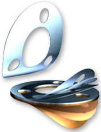
Example of dual composition: a shim of total thickness 1 mm consisting of 8 leaves of 0.1 mm and 4 leaves of 0.05 mm. The exclusive colouring of the metal immediately identifies 0.05 mm leaves in yellow and 0.1 mm leaves in blue
